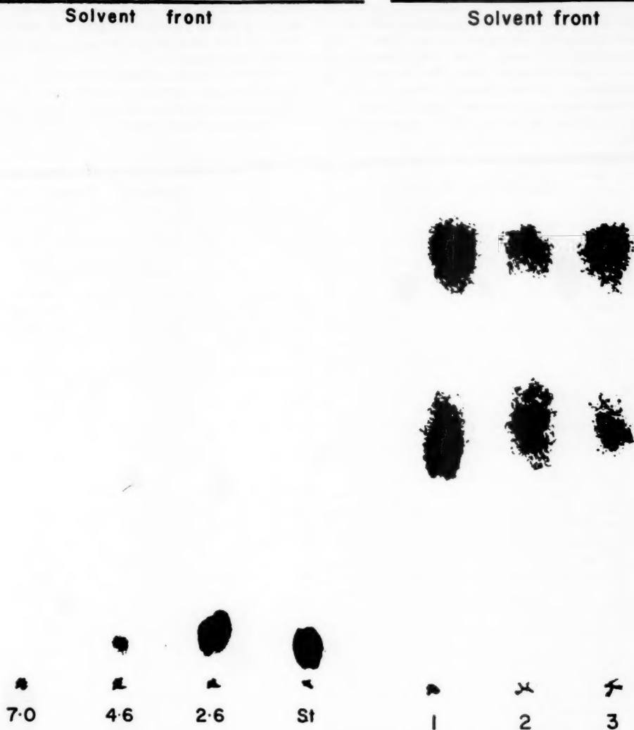
FIG. 1 ( left ). Paper chromatogram of ether extracts of tryptophan treated pea epicotyls. Developing solvent isopropyl alcohol-concentrated ammonium hydroxide-water solvent (80:10:10, v/v). The chromatogram was sprayed with Ehrlich's reagent ( p -dimethylaminobenzaldehyde) in alcohol-aqueous HCl. Numbers refer to the extraction pH. St. is synthetic indoleacetylaspartic acid. Extracts from 3 gm fresh weight of epicotyl tissue were applied to the chromatogram.
